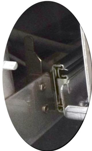
Open the lock of the pull-out mechanism on the right.
