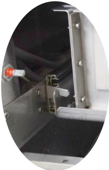
Close the lock of the pull-out mechanism on the right
