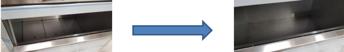
3. Thoroughly rub all storage container walls with a cloth soaked in WESSAMAT special cleaner so that all dirt and limescale residues are removed. Rub thoroughly with clear water to remove all cleaner residues.
